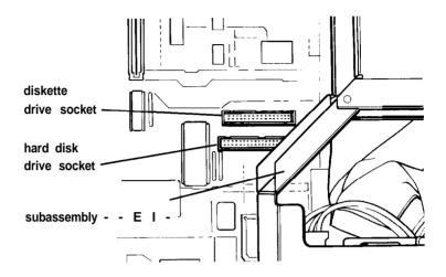
Both sockets have a notch on one side. Connect the diskette drive cable first. As shown below, there is a tab on one side of the connector.
